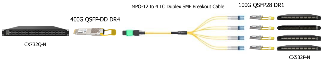
Figure 3 Connect 1 x 400G-port switch to 4 x 100G-port switches
