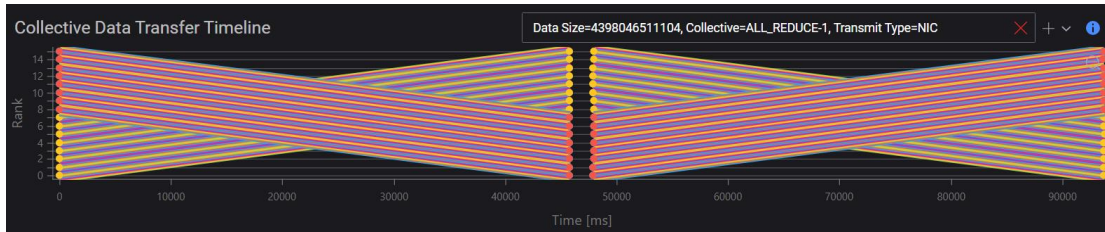
Picture 3-31 2 Nodes x 8 GPUs Spine-Leaf INT-Driven Adaptive Routing All-Reduce Halving Doubling Collective Data Transfer Timeline
