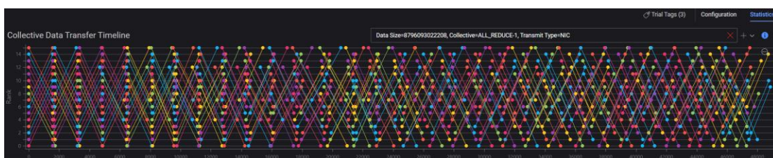
Picture 3-19 2 Nodes x 8 GPUs Spine-Leaf ECMP 5-Tuple Hash All-Reduce Bidir Ring Collective Data Transfer Timeline
