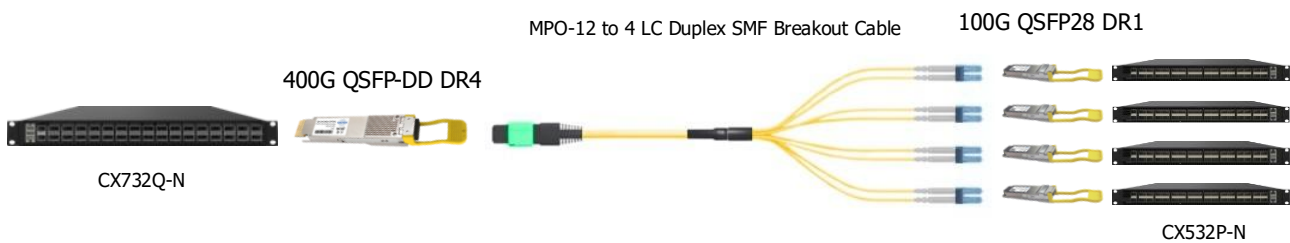
Figure 3 Connect 1 x 400G-port switch to 4 x 100G-port switches
