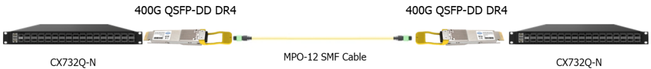
Figure 2 Connect two 400G-port switches
